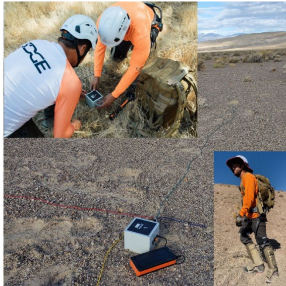
Figure 3. The 3DGE data logger. A tech is shown with a 6-station pack, snake chaps and exoskeleton. Two techs (only one is required) are shown aligning the instrument with magnetic north and setting it level to within 2 degrees using a bubble level. Credit: 3D Edge, Inc., AGB Seismic, LLC and Ashlyn Kudransky Photography.
