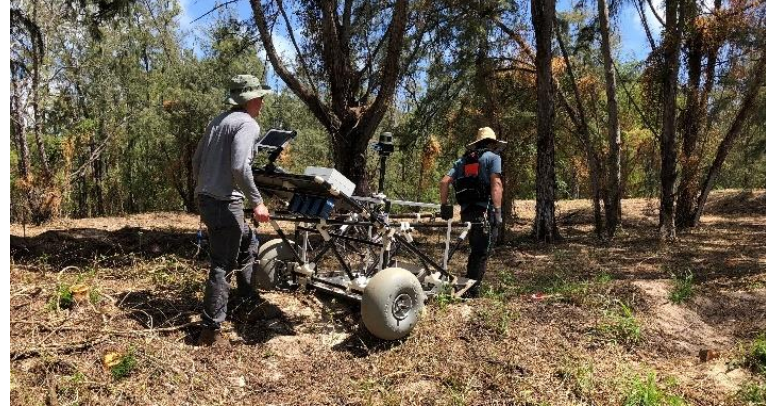
Figure 5: The APEX hybrid cart/litter system configuration is designed for operations in difficult conditions.
