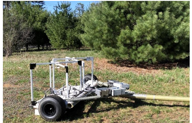
Figure 6: Modular and scalable, the APEX units can be linked to build wider towed arrays for operation in relatively flat, open sites. The scalable architecture allows for building arrays of N units. Several projects are planned in 2024 for towed arrays comprising as many as 3 to 4 units per towed system, enabling high production rates.
