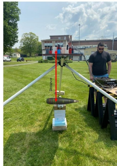
Figure 7 - ULEMA-R Detection depth for a horizontal 155 mm projectile horizontal in test-stand. The noise floor is shown for comparison (left). The test stand set-up is shown as well (right).
