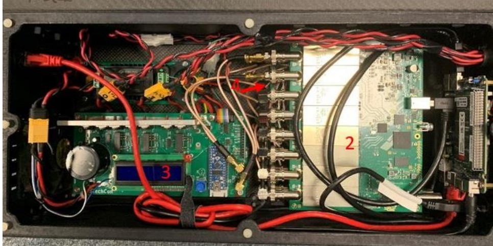
Figure 2 - ULEMA Electronics Box. The major components are (1) the brick computer running the software, (2) the Field Programmable Gate Array (FPGA) handling the incoming data and the outgoing current, (3) the transmitter board sending out the pulsed current, controlling the on and off times which allow for the decaying secondary field to be detectable, and (4) the amplifier boards, which increase the incoming data magnitude to make the responses better distinguishable, positioned directly below the FPGA.
