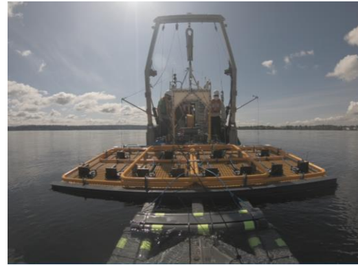
Figure 1. Left: sensor geometry of the UltraTEM: four horizontally arranged transmitters and twelve triaxial receiver cubes. Right: View of the UltraTEM and Ugly Duckling vessel from a camera mounted at the stern of the tow-fish. This photograph was taken at Lake Washington.
