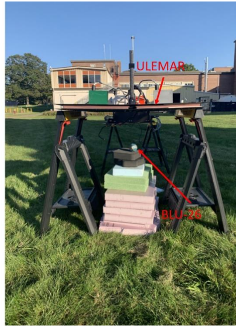
Figure 8 – ULEMAR Detection depth for BLU-26 submunition, with noise floor for comparison (left). The test stand set-up is shown as well (right).
