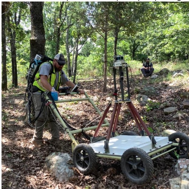
Figure 3: Temsense data collection with Stencil SLAM positioning
