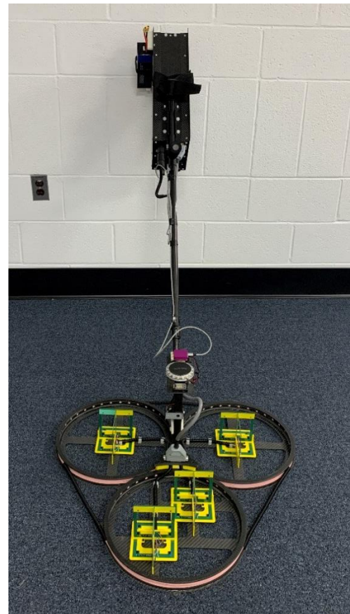
Figure 1 - View of ULEMA Array Configuration. The direction of travel is defined along the axis of symmetry of the system, with the transmitter in the front.
