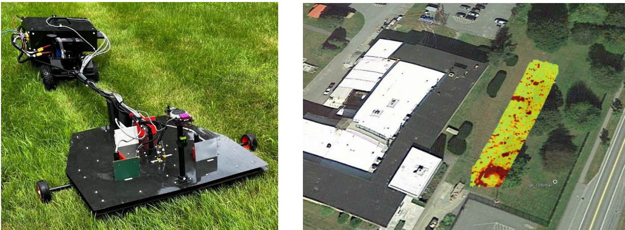
Figure 6 - ULEMA-R during the data collection (left). ULEMA-R EMI detection map overlaid on the Google map (right).
