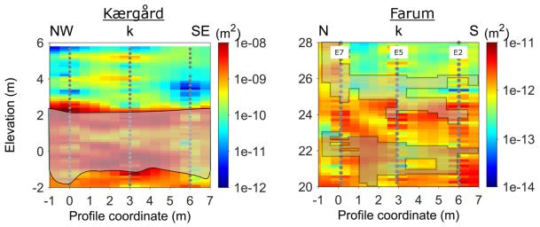
**Figure 3.** Permeability models obtained from cross-borehole DCIP inversion at Kærgård (left, published by Bording et al., 2021) and Farum (right). Note the different colour scales. The shaded grey zone indicates the distribution of the low-resistivity anomaly (all cells with a resistivity ratio lower than 0.3) along the profile at +1 day for Kærgård and +270 days for Farum. Electrodes are indicated by grey filled circles.
