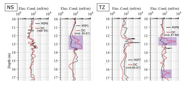
**Figure 2.** Comparison of "true" electrical conductivity measured by induction logs (MIP1, MIP6, MIP7 and MIP8, see location in Fig. 1) with inverted conductivity from cross-borehole ERT at Inj#2+20 days in Farum. The depth range 10-20 m corresponds to elevation range 19-29 m.
