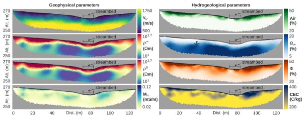
**Figure 2** Subsurface models resolved through the proposed PJI schemes. The black dots indicate the sensor/shot positions. The groundwater level observed in a borehole nearby is indicated in the resolved saturation model. (a) Subsurface air content, saturation and porosity. (b) Estimation of both  $\rho^{\infty}$  and  $\rho^{0}$  permits the computation of the normalized chargeability  $M_n$ . Additionally, the CEC is obtained through the application of this PJI scheme.
