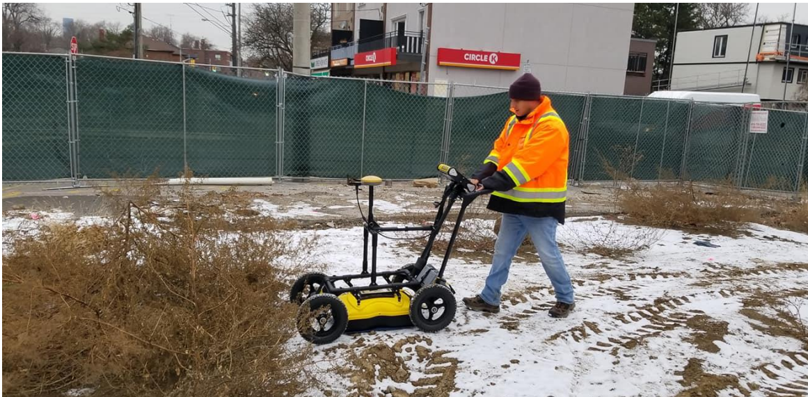
Figure 1: Photograph facing west of GPR data acquisition at the project site.
