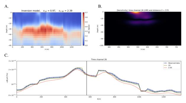
*Figure 1* A. Inversion model obtained with quasi-2D inversion. B. The sensitivity to a data point at 570m and 0.1722 ms. C. Comparison between the observed data  $\mathbf{d}^{obs}$ ,  $\mathcal{F}_{1D}(\mathbf{m})$  and  $\mathcal{F}_{2.5D}(\mathbf{m})$ .
