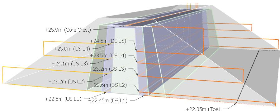
**Figure 1** Cable layout in the Test Dam.
