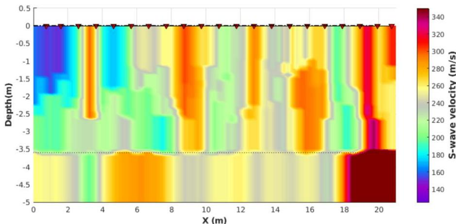
**Figure 2**  $V_s$  model obtained from the first phase of analysis.
