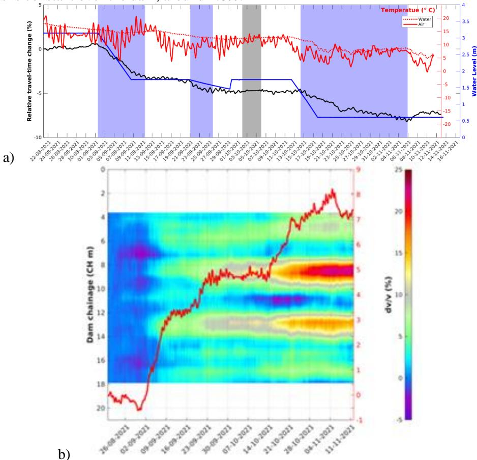
**Figure 3** Monitoring results for Phase 2. a) average travel time variations (black line) with water temperature (dotted red line), air temperature (red line) and water level measurements (blue line). b)  $dv/v$  measurements along the dam. The red line shows the average  $dv/v$  throughout the dam.
