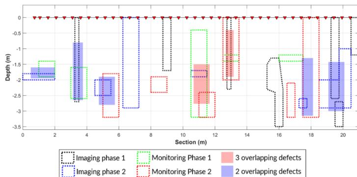
**Figure 4** Defect identification summary. Areas of velocity anomalies identified by both the imaging and monitoring and/or during both monitoring phases (the blue and pink shaded areas).
